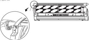
Secure either the upper or lower edge of the air inlet panel by lightly pushing it in, and then close the panel.
