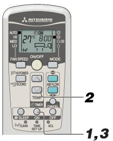
Example: In the case you wish to bring the temperature to nearly set temperature in at 8:00. Aim the remote control at the air-conditioner.
