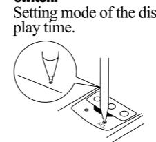
When the indicator shows any abnormal condition,press the reset switch with the tip of a ballpoint pen.
