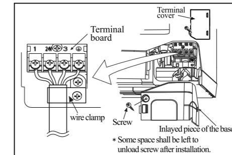
Use cables for interconnection wiring to avoid loosening of the wires.
