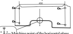
Four screws are used to horizontally adjust the installation board when it is under the temporary fastening status.
