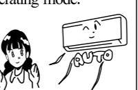
The Auto mode automatically selects the operation mode (HEAT, COOL or DRY), depending on the room temperature when switched on.
