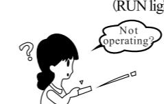
Restarting has been blocked for 3 minutes after you have stopped, to protect the unit.
