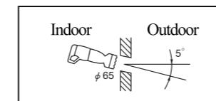
The core drill is used for drilling
